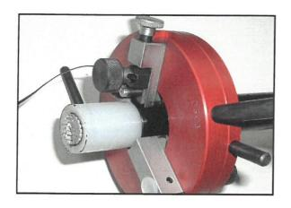
Adjust the correct cutting depth of the shaving blade.
