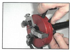
Fix the tool on the cable. All 3 sliding parts must touch the surface.
