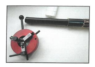
Straighten the cable, clean surface and use silicone grease.
