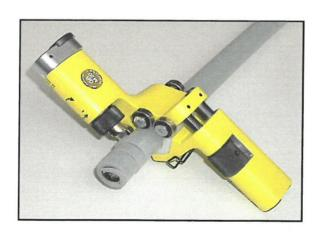
Use the Sheath Stripper **GB-M20** to cut and remove the isolation.
