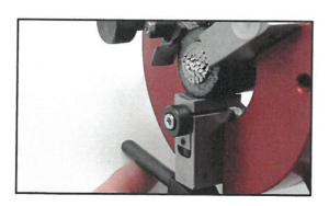
Place forward the lever. So this sliding part is under spring tension.
