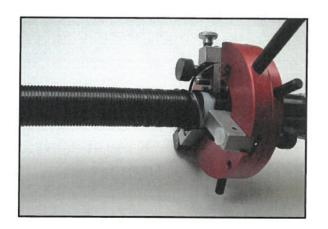
Circular Cut si made when the tool is reaching the stop rings.
